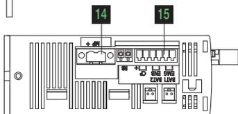
**1 Motor connector for axis 1**
